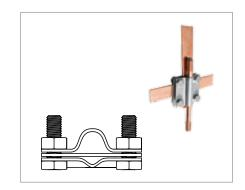
Cruciform clamp – profile, bolted M8 with stainless steel separator, to connect rod to galvanized tape or circular conductor (with stainless steel separator inside protecting from corrosion between copper and zinc when different metals are connected)
